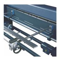
A cost-effective solution for simple applications that do not require frequent readjustment. Hand stops are equipped with the rack - pinion system and the position indicator, which the operator can adjust
